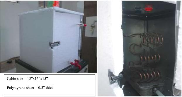
Fig 1.3 Insulated polystyrene cabin having copper tubes and hot water sink
