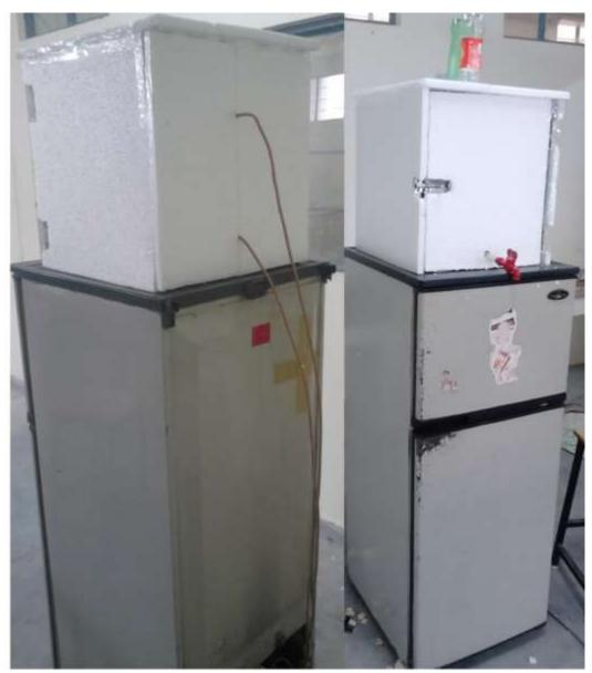
Fig. 1.2 Waste heat recovery system from domestic refrigerator
